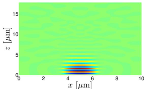
Grating dimensions tuned to reflection at  $\lambda = 1.55 \mu\text{m}$ .
